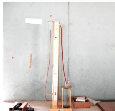
Plate 3: Jecon Void or Porosity Meter
