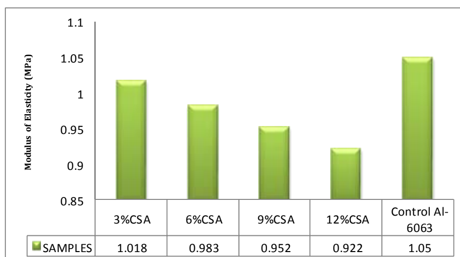
Figure 8. Shows the variation of Modulus of Elasticity for the control sample and reinforced AA6063/CSA composite
