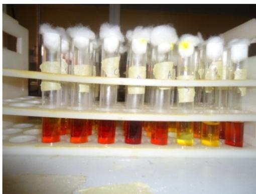
**Figure 5.** The use of DNS reagent to test for the presence of reducing sugars
