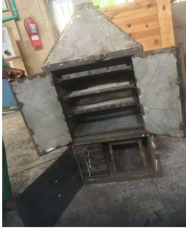
Figure 3. Fabricated multi-source powered oven
