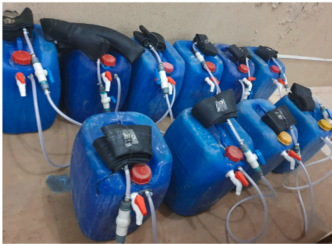
Fig. 2. 25 liters anaerobic digester.
