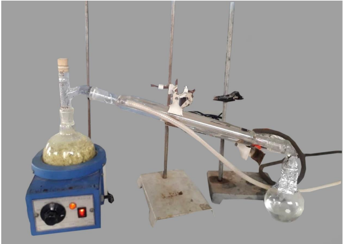
Plate 1: Simple distillation apparatus used for extracting essential oil from lemon and lime
