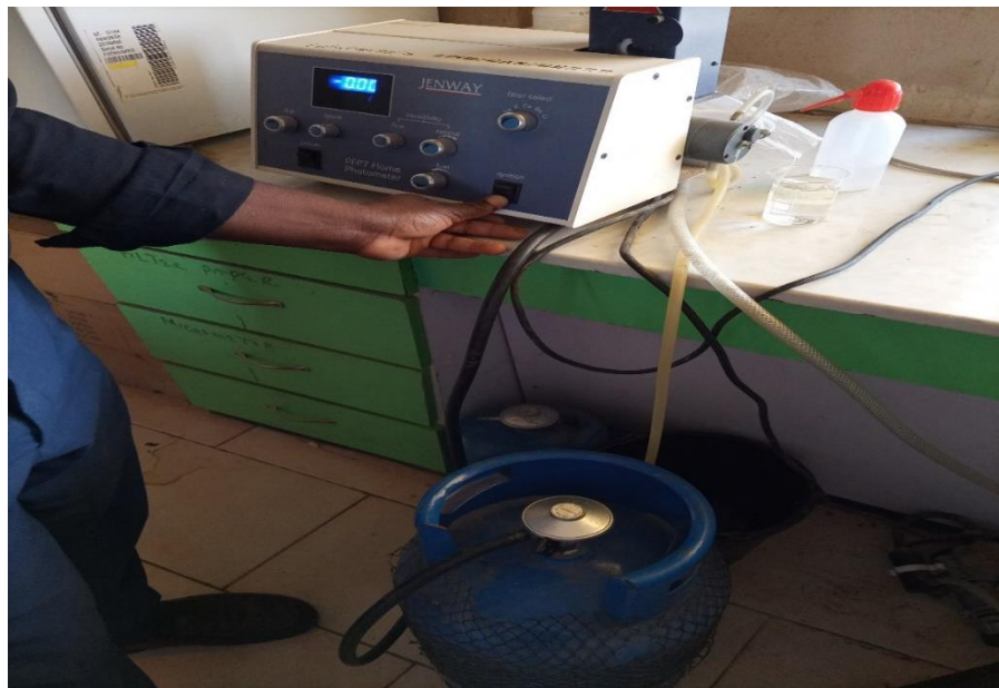
Plate 3.3: Flame photometer apparatus used to analysis Na, Mg Concentration.
