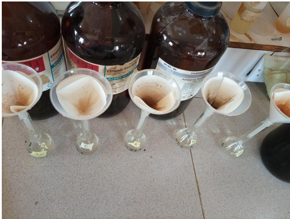
Plate 3.4: Filtration process during acid digestion of soil samples.
