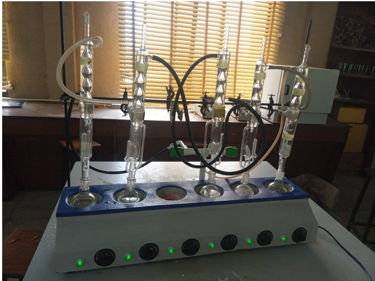
Plate 3.1: Oil extraction using Soxhlet's apparatus.
