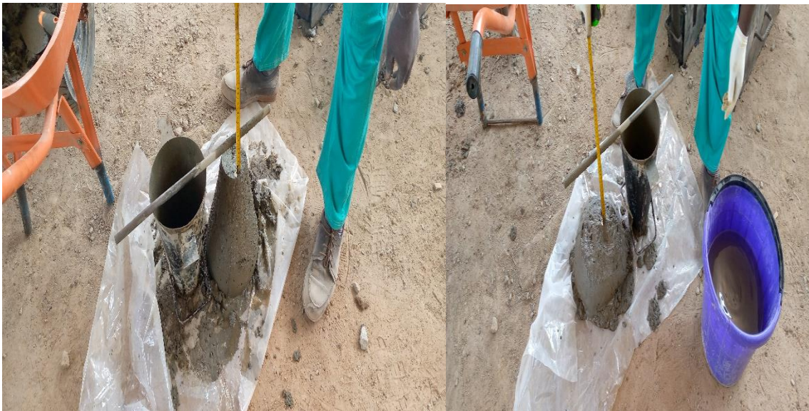
Figure 3.9c-d: Slump test for different percentages of CPA
