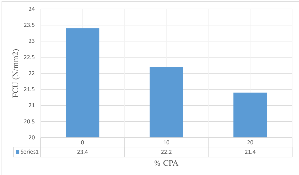
Figure 4.7: Compressive strength test result
