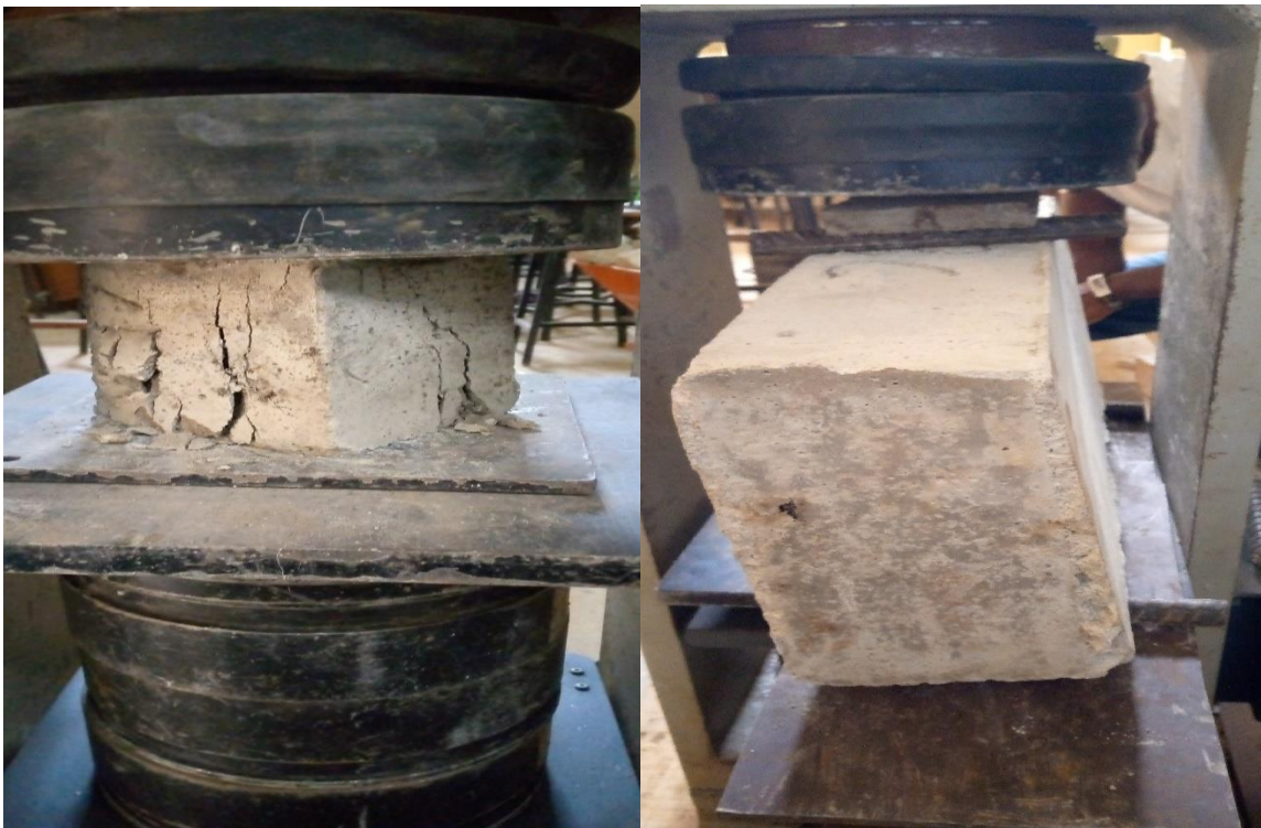
Figure 3.11a: Crushing of beams and cubes
