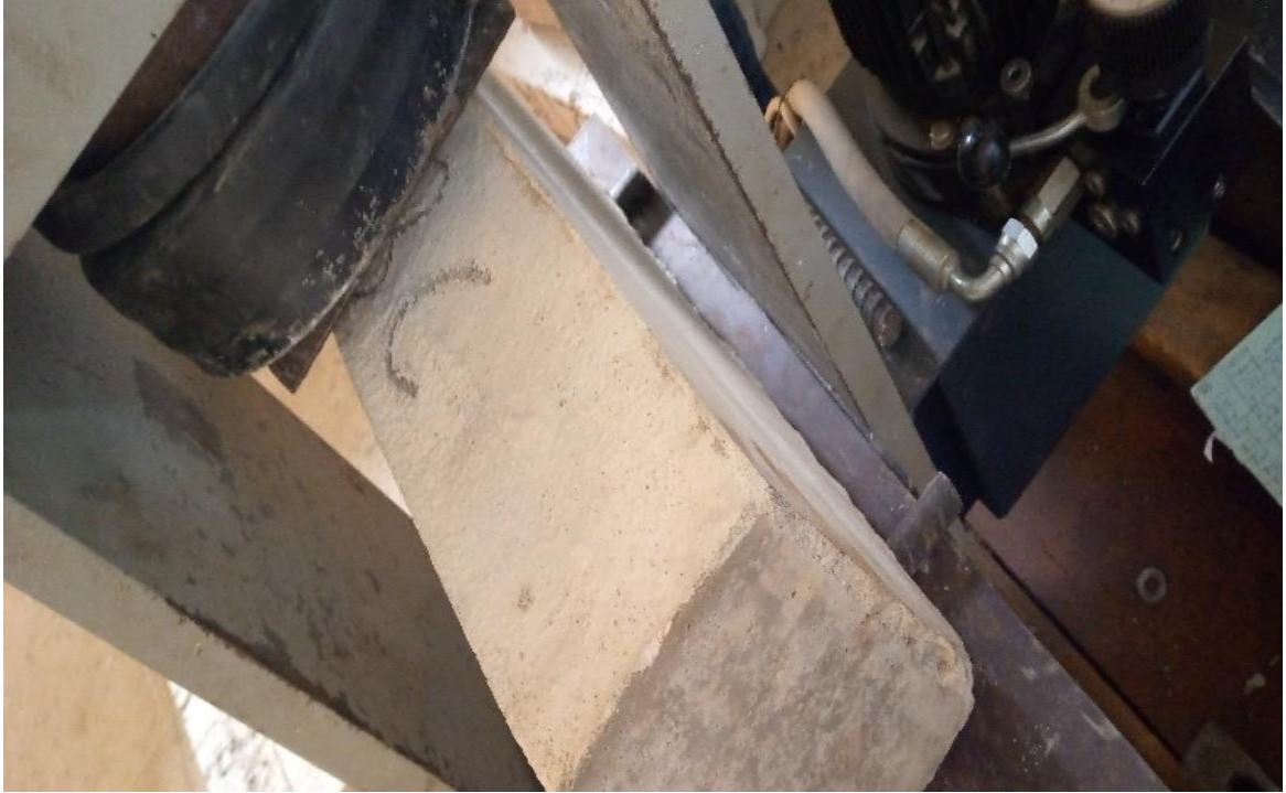
Figure 3.11b: Crushing of beams and cubes
