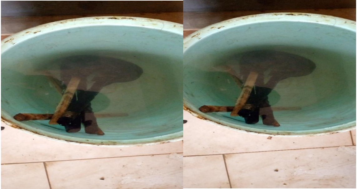
Figure 3.7: Water Absorption test on bamboo
