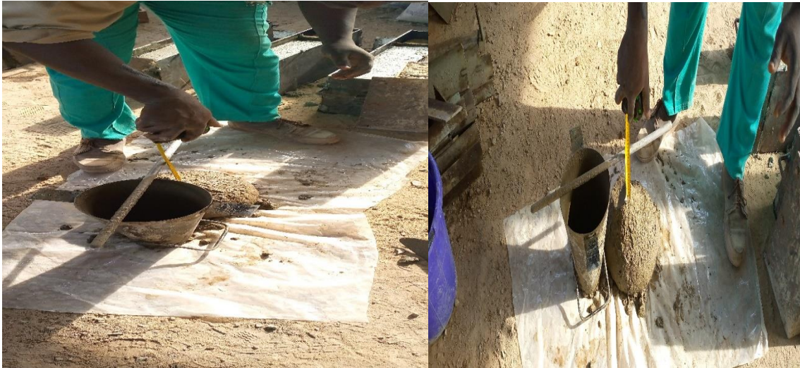
Figure 3.9a-b: Slump test for different percentages of CPA
