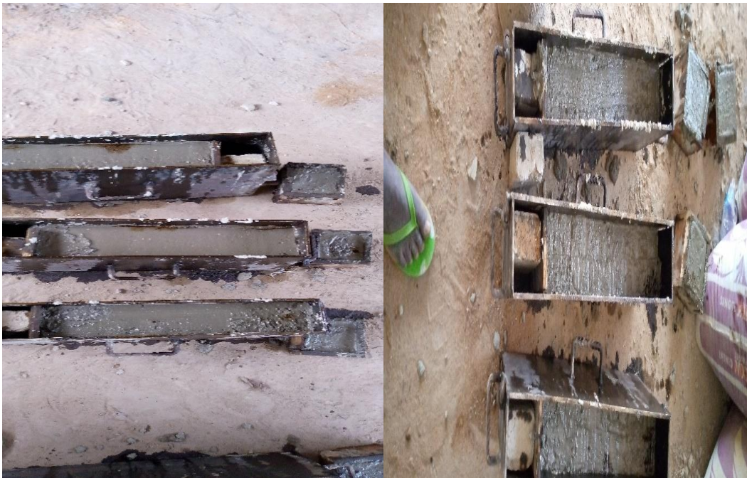
Figure 2: Already mixed concrete poured into moulds
