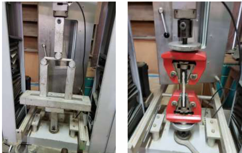
Fig. 2 Mechanical Tests on samples, a Test on Modulus of rupture, b Test on modulus of elasticity
