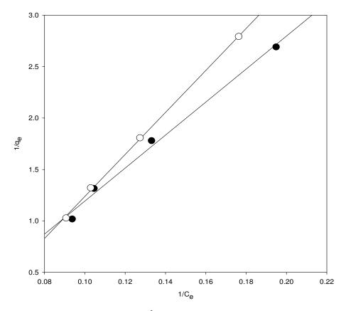
Figure 2. Langmuir isotherm for  $Cr^{6+}$  by (open circles) PAEI and (closed circles) PAEB.
