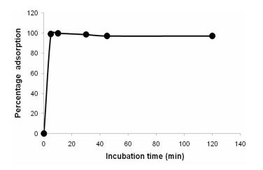
**Figure 1.** Dependence of contact time of adsorption of Pb(ii) ion by EBAO.
