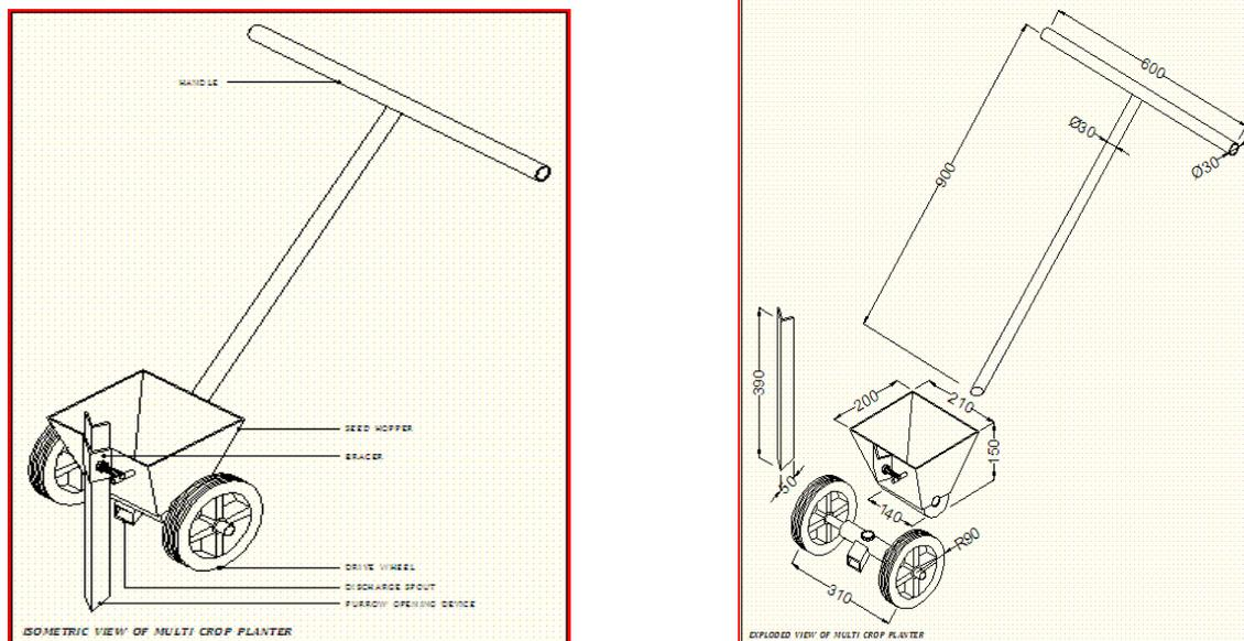
**Fig. 1:** Isometric and exploded views of the planter
