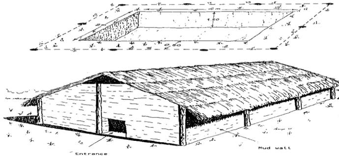
Figure 6: The Thatched-roof Pit or Cellar-hut Storage Structure. Source: MFCL, GMC & NARI (2004)
