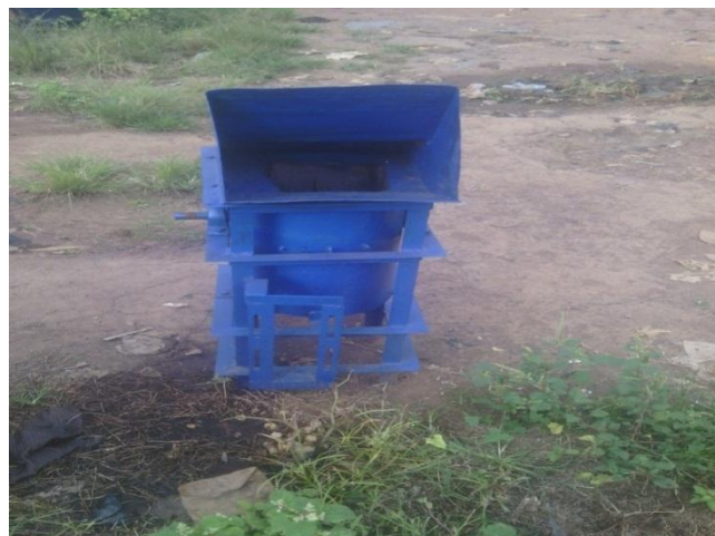
Fig.-4 Manufactured horizontal shaft impactor crusher
