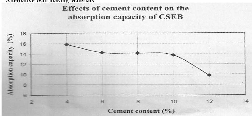
Fig. 8 Effects of cement on the absorption capacity of soil cement block.
