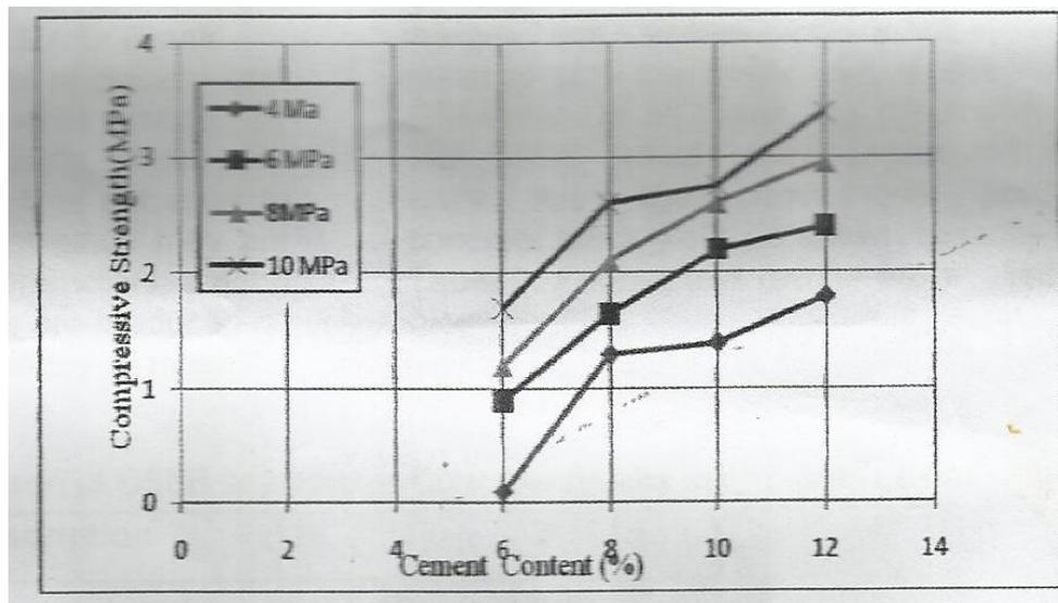
**Fig.7:** Effect of compaction pressure on compressive strength of CSSB
