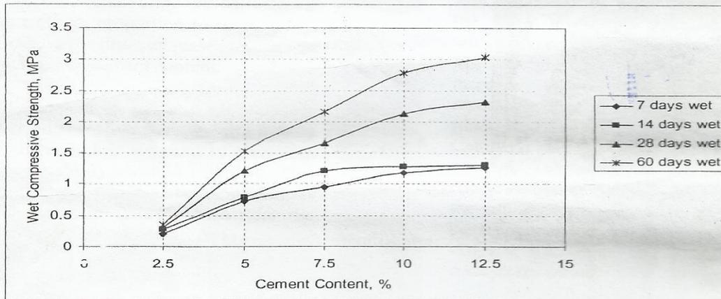
Fig. 4 Effect of Cement Content and Curing on Compressive Strength
