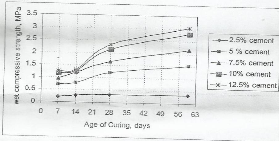
Fig. 6 Effect of Age of Curing on Compressive Strength
