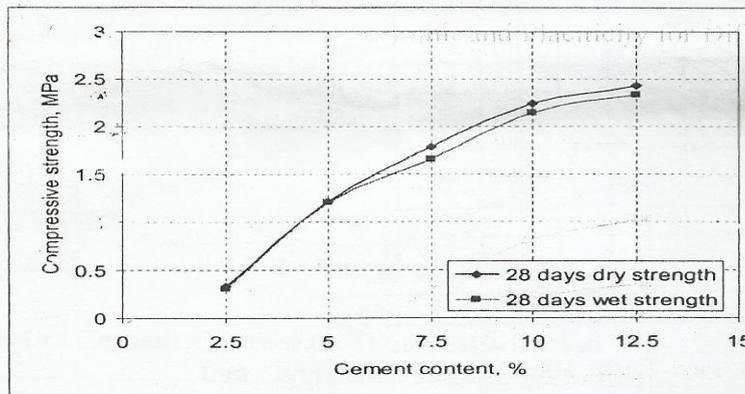
Fig. 5 28 Days Wet and Dry Strengths of Specimens
