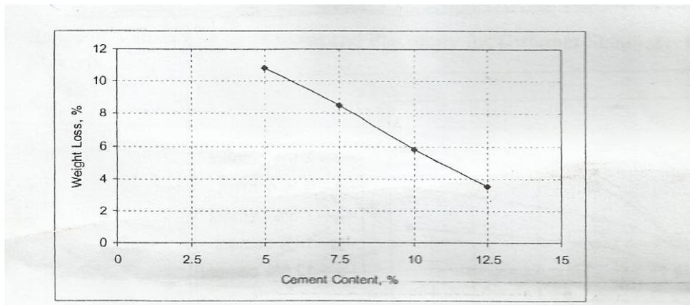
**Fig.9 Effect of Cement Content on Durability**
