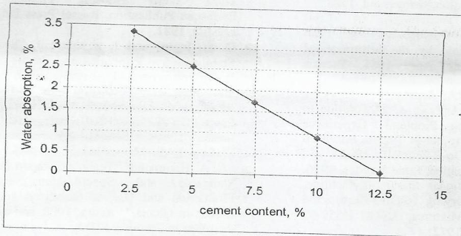
Fig.7. Effect of Cement Content on Water Absorption
