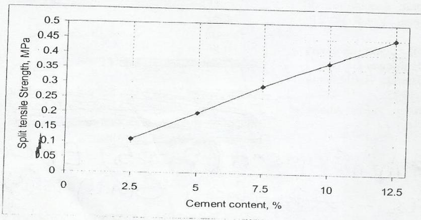
Fig.8 Effect of Cement Content on Split-Tensile Strength
