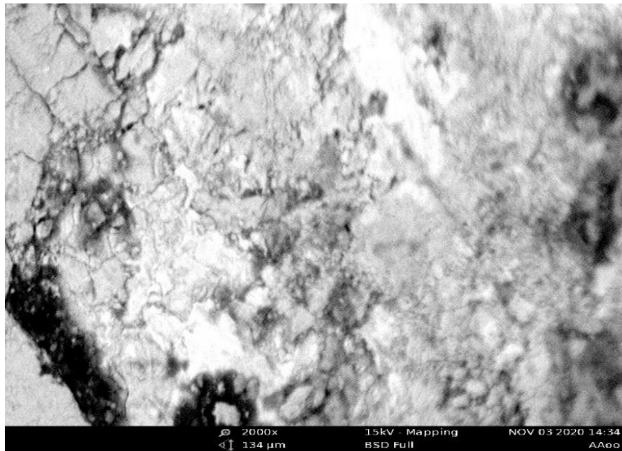
Figure 6. SEM micrograph for Blank MS coupons.
