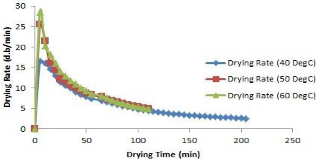
Figure 2: Graph of Drying Rate versus Drying Time for the drying of fish cracker
