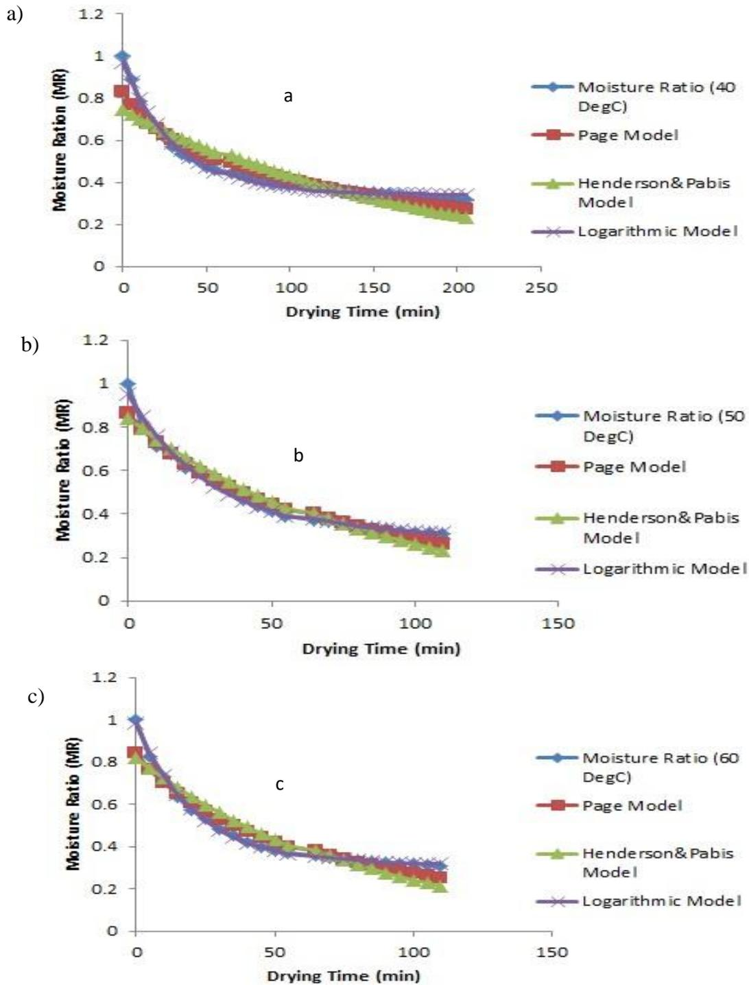
Figure 3: Prediction of experimental moisture ratio as a function of drying time using thin layer semi empirical drying models at (a) 40 °C (b) 50 °C (c) 60 °C.
