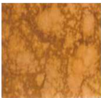
Figure 2: Optical macrograph of metal side of manganate coated specimen after adhesion test.
