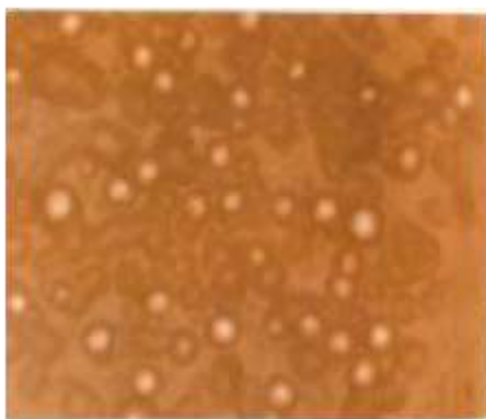
Figure: 3 optical macrograph of tape side for manganate coated specimen after adhesion test.
