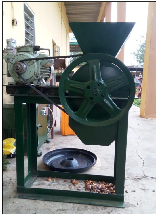
Figure 4. Pictorial view of the cocoa depodding machine
