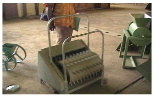
Plate 1: NCAM Pedal Operated Thresher
