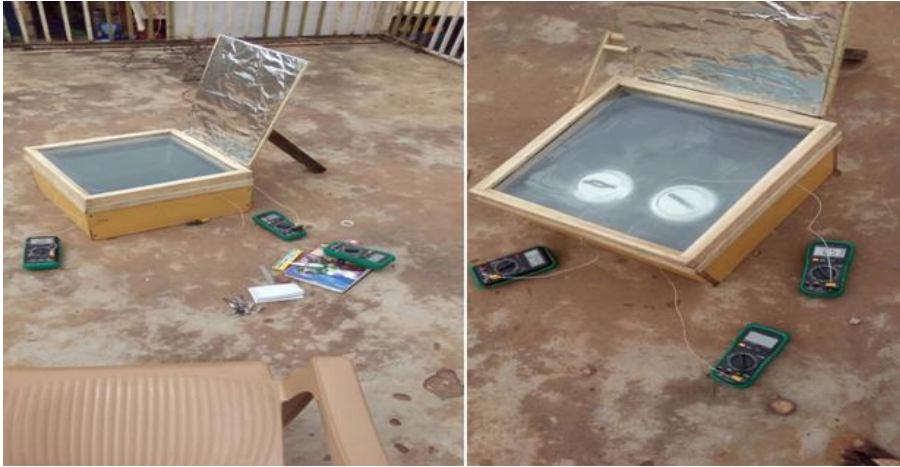
Plate 1: Setup of the Solar Box for stagnation and sensible test showing the multi-meters used in measuring the chamber, absorber and water temperatures
