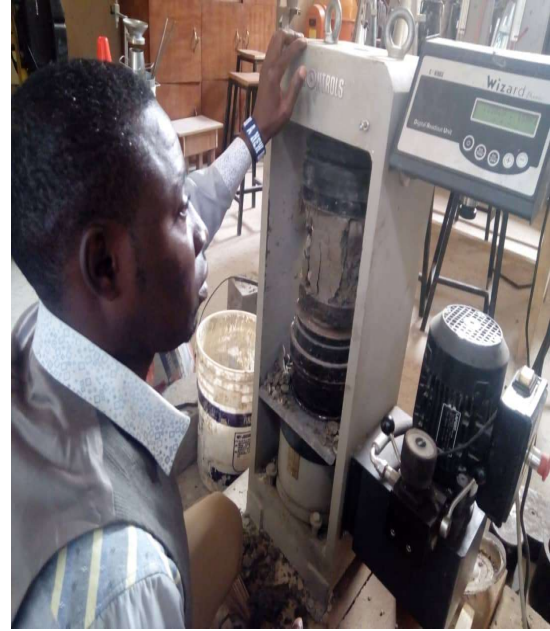
Plate V: Cube crushing test with a digital crushing machine
