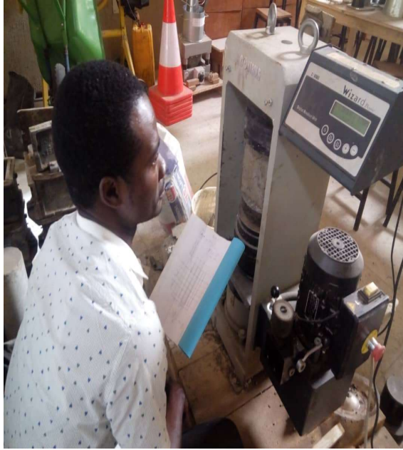
Plate IV: Cube crushing test with a digital crushing machine
