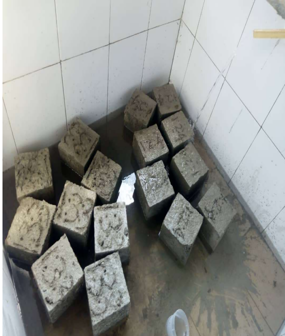
Plate VI: Cube in the curing tank
