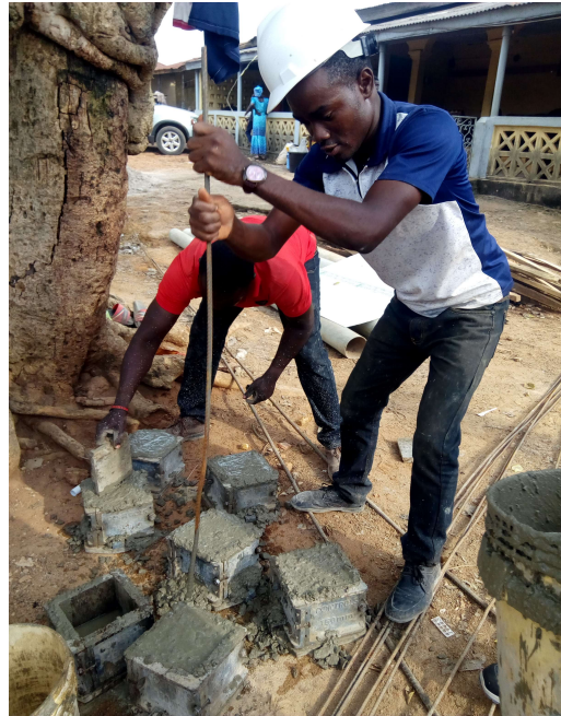
Plate II: Compacting of green concrete in layers
