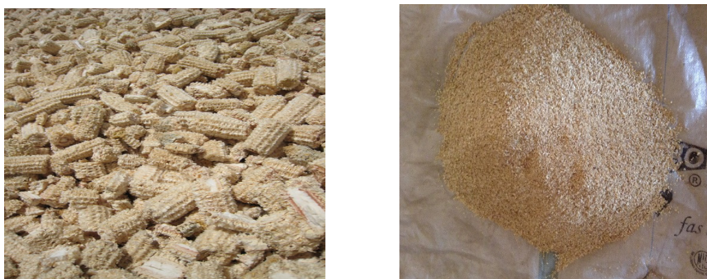
Figure 1 Corncob (a) before grinding (b) after grinding
