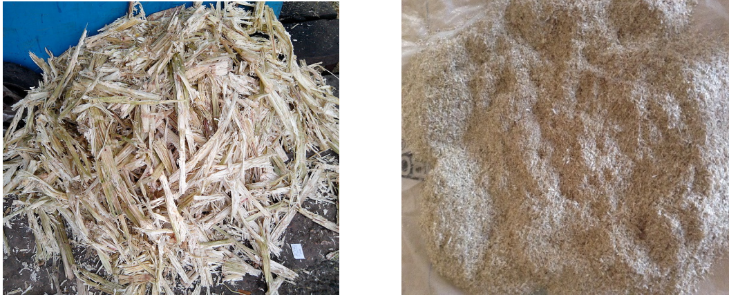
Figure 2 Sugarcane Bagasse (a) before grinding (b) after grinding
