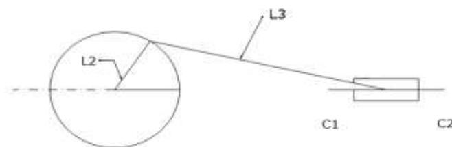
**Figure 9** Crank Slider Mechanism Showing the Maximum Displacements C1 & C2
