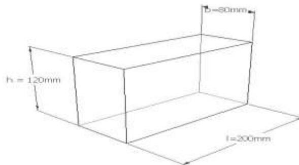
**Figure 6** Isometric view of the Cutting chamber
