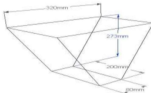
**Figure 3** Isometric view of Exaggerated Hopper
