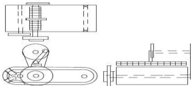
Figure 1 Orthographic View of Plantain Slicing Machine
