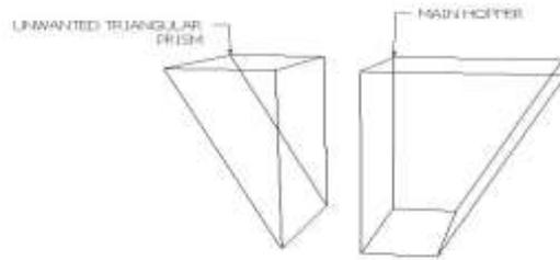
**Figure 5** Isometric view of main hopper separation
