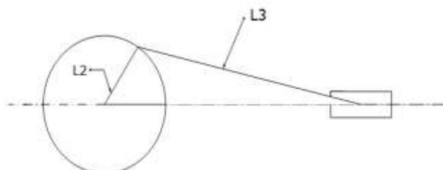
**Figure 7** Crank slider mechanism
