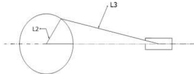
**Figure 7** Crank slider mechanism
