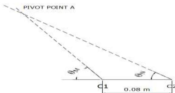
**Figure 8** How to locate the axis of the pin joint C
