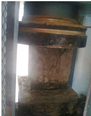
Plate VII: Crushing of cubes using compressive
