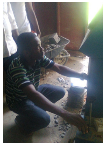
Plate VII: Crushing of cubes using compressive
