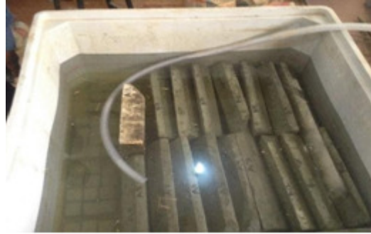
Figure 3 Water curing of samples
