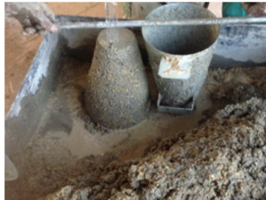
Figure 5: Slump test measurement of samples
