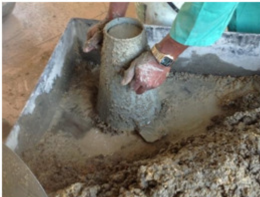
Figure 4 Slump test for samples
