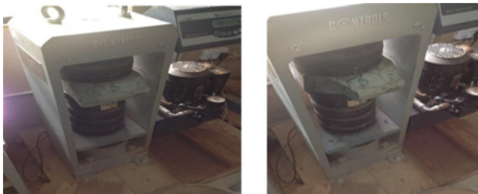
Figure 2 Sample before crushing and after crushing respectively
