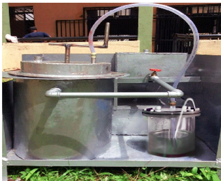
Plate 2. Setup of the designed and constructed anaerobic digester
