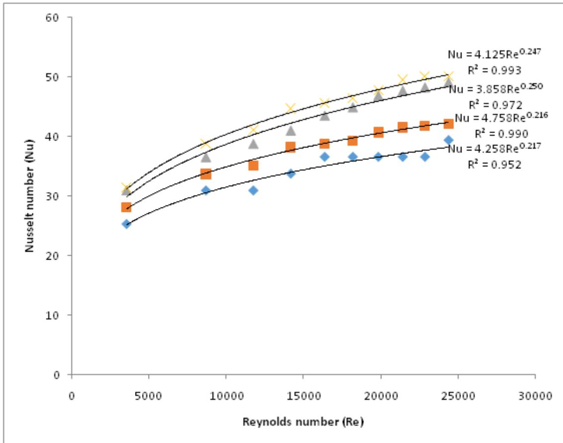
**Figure 4.** Relationship between  $Nu$  and  $Re$  for flow past staggered tube bank
