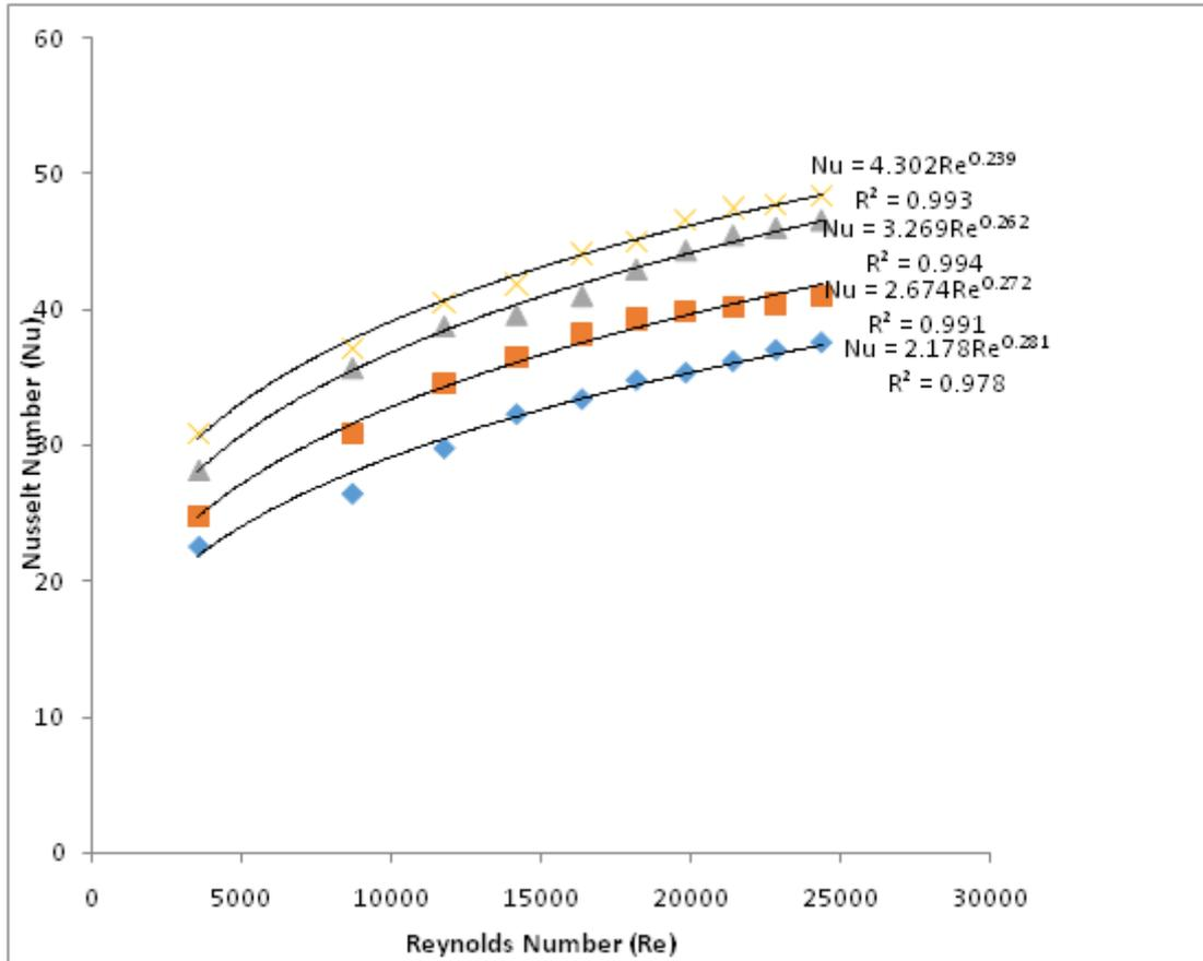
**Figure 5.** Relationship between  $Nu$  and  $Re$  for flow past in-line tube bank
