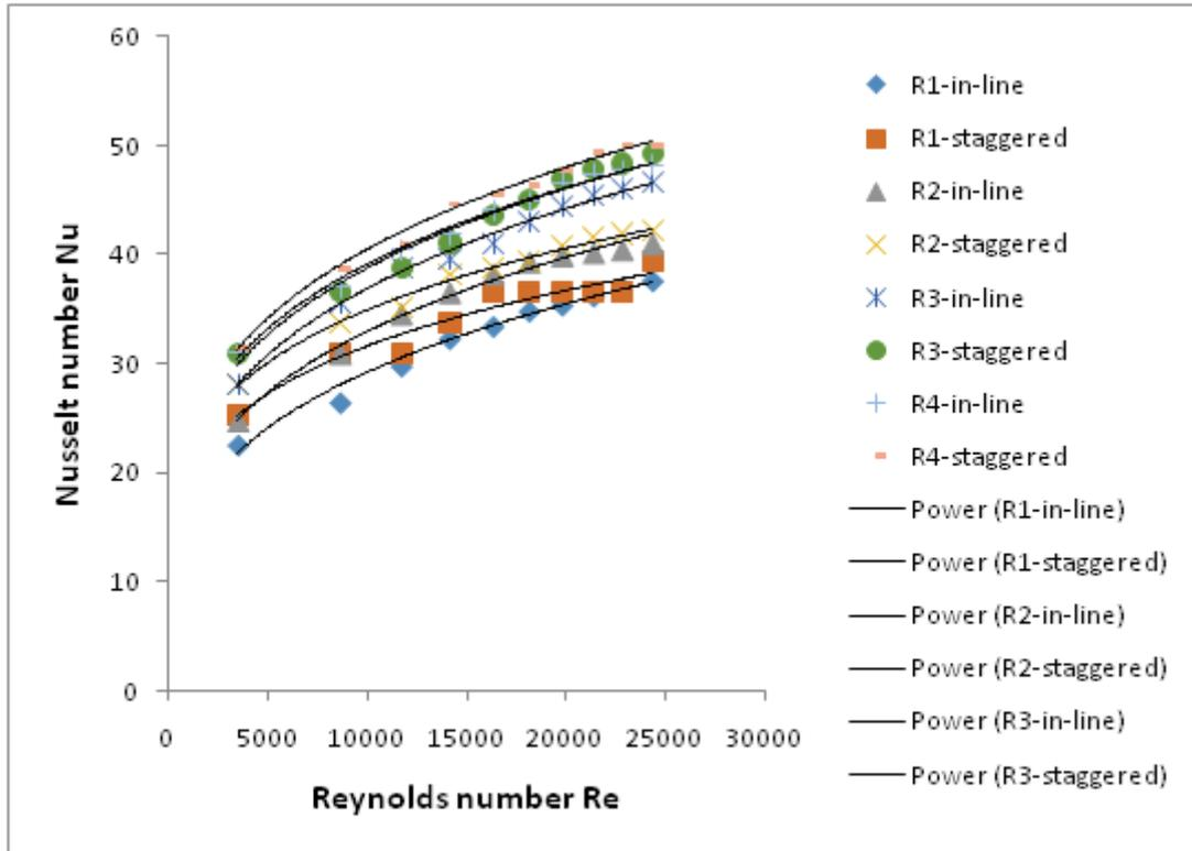
**Figure 6.** Comparison of Nu for staggered and in-line tube banks
