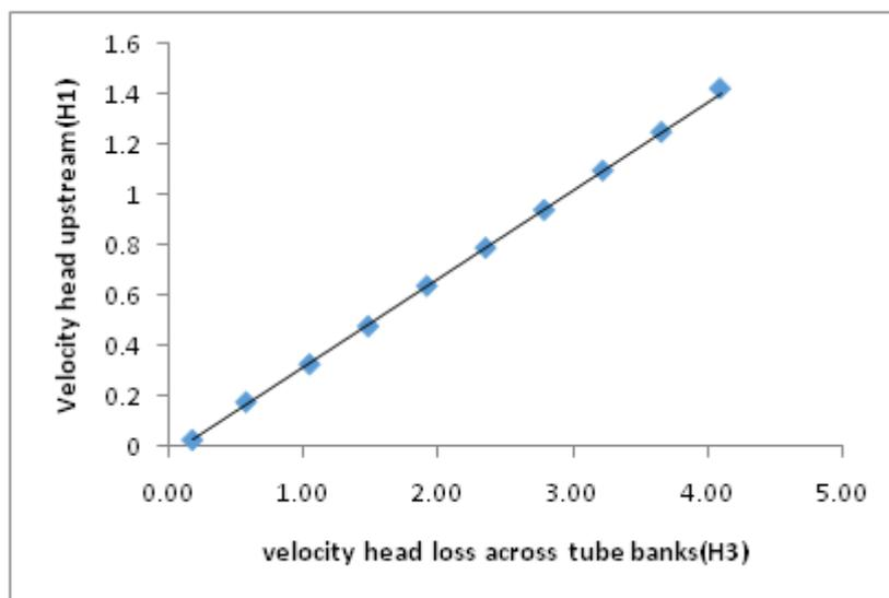
**Figure 3.** Velocity head upstream and velocity head drop across in-line tube bank
