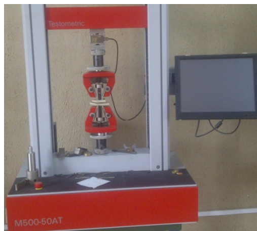
Figure 2. Instron-universal tensile testing machine (M500-50AT)
