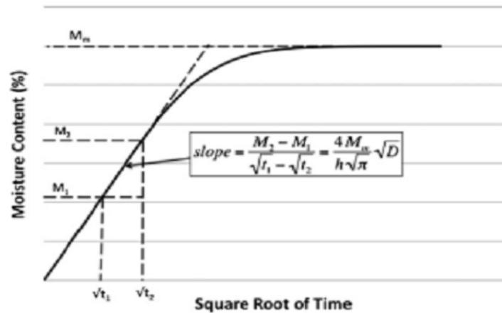
Figure 3: Determination of Diffusion Coefficient (Londhe *et al.*, 2016)
