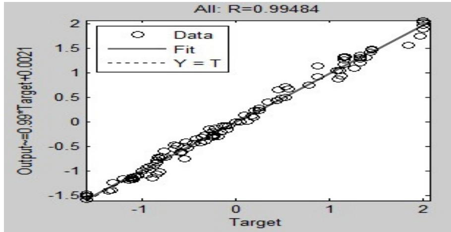
Figure 8 Model Efficiency for 2-5-1-1 Topology
