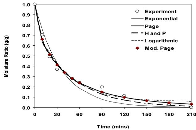
Figure 8. Experimental and predicted moisture ratio for EX-BORNO at 70°C
