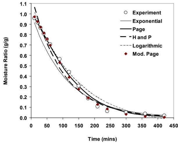
Figure 5. Experimental and predicted moisture ratio for SOSAT C88 at 40°C
