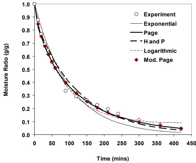
Figure 7. Experimental and predicted moisture ratio for EX-BORNO at 40°C
