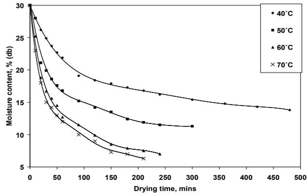
Figure 2. Drying curve for EX-BORNO millet
