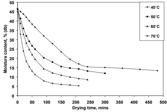
Figure 1. Drying curve for SOSAT-C88 millet
