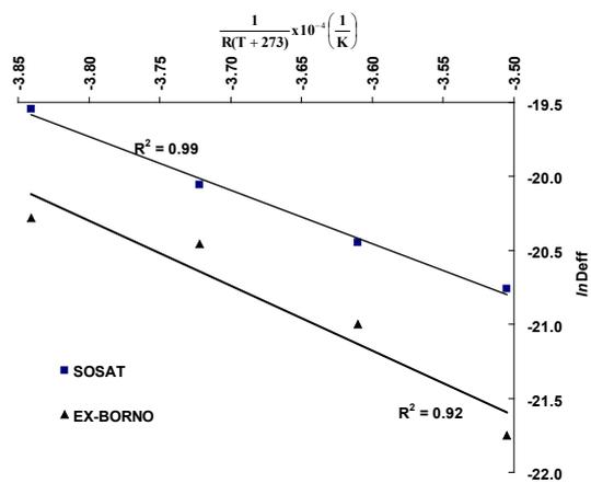
Figure 9. Arrhenius-type relationship between effective diffusivity and temperature.
