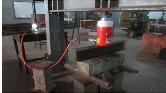
Fig. 2. Set up of flexural strength test on beam.
